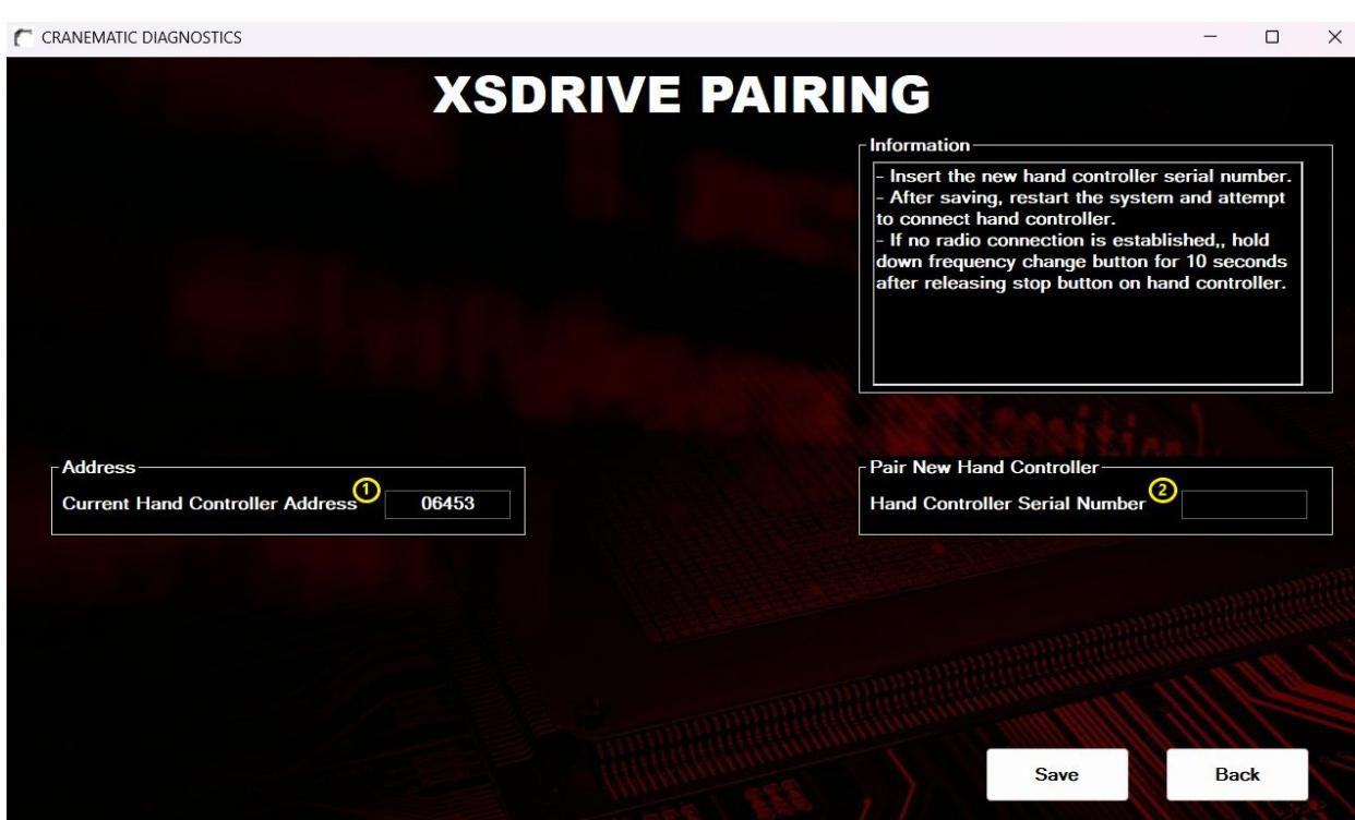
① **Current hand controller address** - Displays the address of the currently paired hand controller. This address can be found on the identification label on the remote controller.
