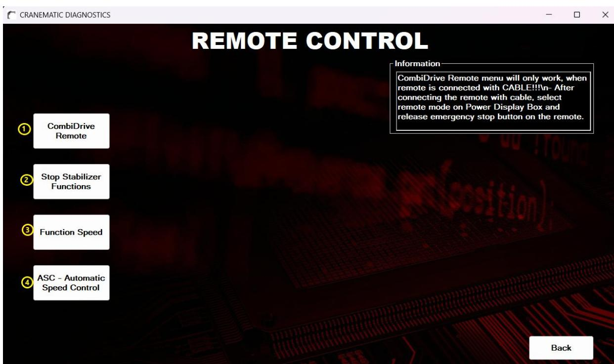
① **CombiDrive Remote** - Assign functions to buttons, configure additional controls, and enable special features.
