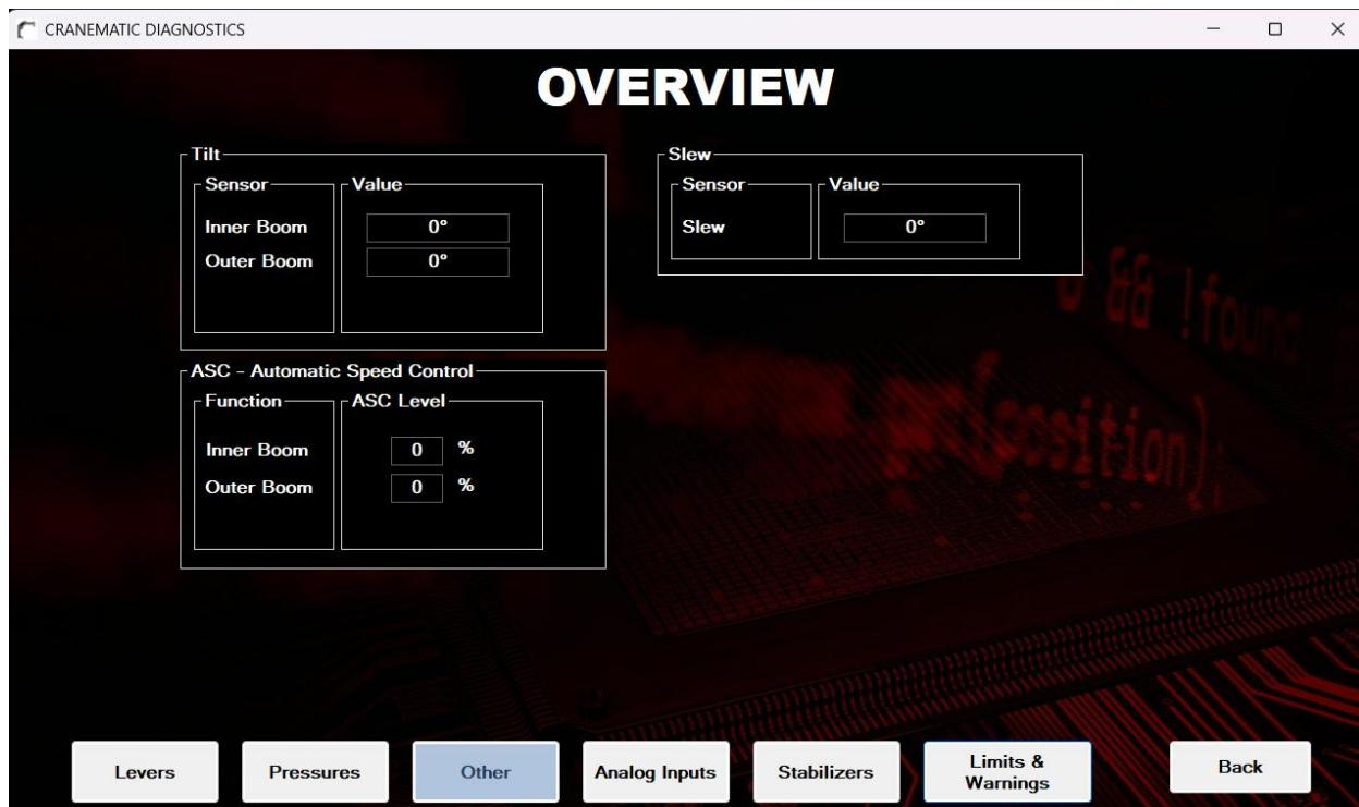
Displays an overview of all other sensor values in the system, providing a real-time view of sensor inputs used by the control unit.
