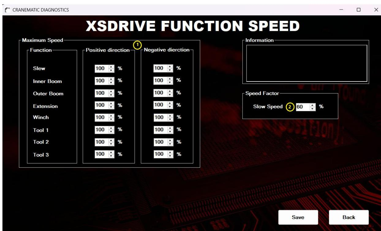
① **Function maximum speed limits** - Defines the maximum operating speed for each function, configured separately for both movement directions.
