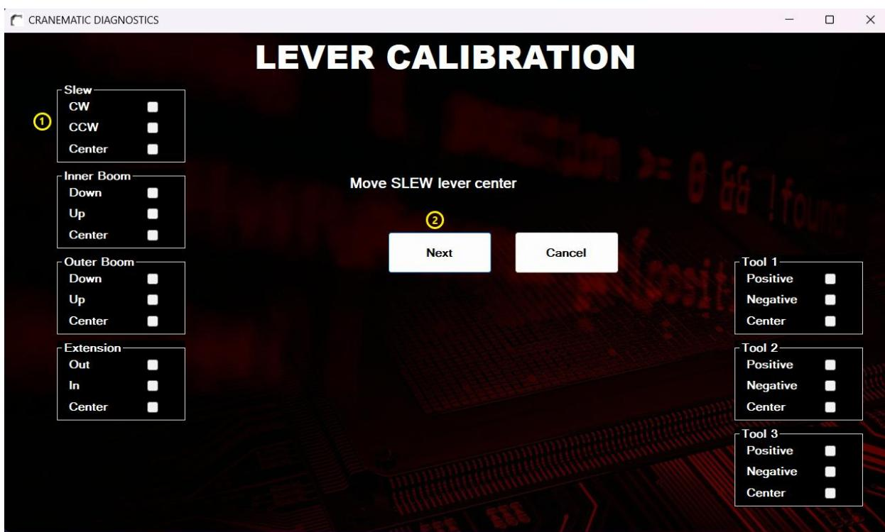
① **Calibration progress** - Each calibration step is marked as completed once the required action has been successfully performed.
