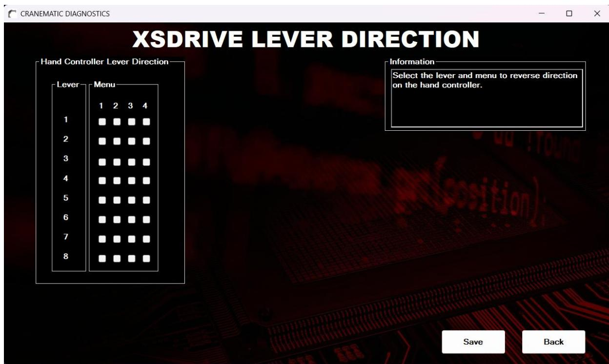
Select the lever and the menu for which the remote lever direction should be changed. This allows the control direction to be adapted to the selected menu or operating situation, ensuring intuitive crane operation.
