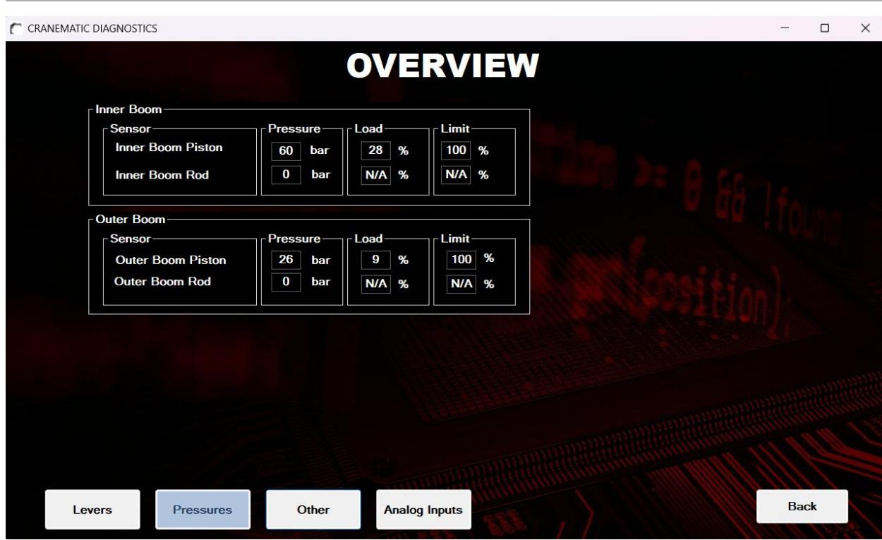
Displays an overview of all pressure sensors in the system, including current pressure values, calculated loads, and configured pressure limits.
